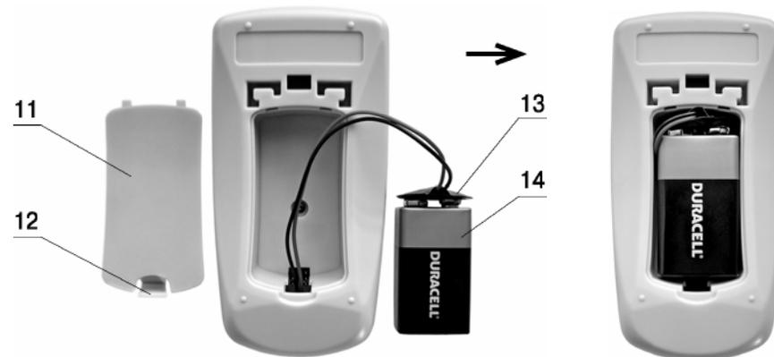
Figure 2 – Power battery mounting
